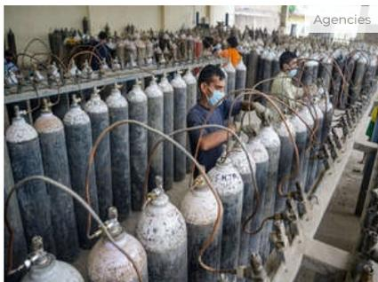
Oxygen produced at on-site plants has to be compressed and filled in cylinders/special vessels using high pressure compressor for transporting to hospitals.
